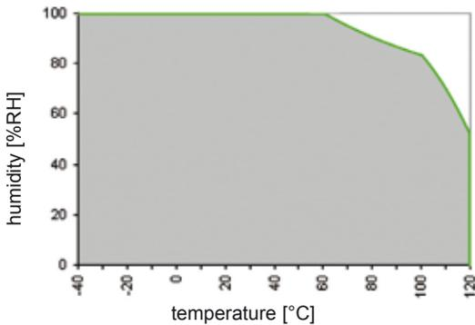
The working range of the humidity sensor element is shown in terms of humidity / temperature limits.
