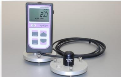
The AL-100 leveling plate is recommended for use with the MU-200. To facilitate mounting to a cross arm, the AM-110 mounting bracket is recommended for use with the AL-100.
