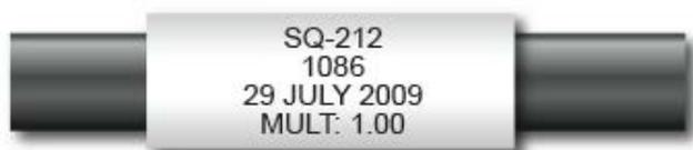
Sensor model number, serial number, production date, and calibration factor are located near the pigtail leads on the sensor cable.
