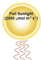
Example of PPF measurement with an Apogee quantum sensor. Full sunlight yields a PPF on a horizontal plane at the Earth's surface of approximately  $2000 \mu\text{mol m}^{-2} \text{s}^{-1}$ . This yields an output signal of 4000 mV for the 0-5 V option or an output signal of 2000 mV for the 0-2.5 V option. The signal is converted to PPF by multiplying by the calibration factor.
