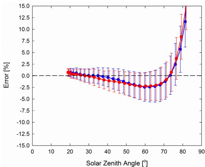
Mean cosine response of twenty-three SQ series quantum sensors (***error bars represent two standard deviations above and below mean***). Cosine response measurements were made by direct side-by-side comparison to the mean of four reference thermopile pyranometers, with solar zenith angle-dependent factors applied to convert total shortwave radiation to PPF. Blue points represent the AM response and red points represent the PM response.
