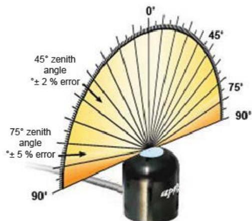
Directional, or cosine, response is defined as the measurement error at a specific angle of radiation incidence. Error for Apogee SQ series quantum sensors is approximately  $\pm 2\%$  and  $\pm 5\%$  at solar zenith angles of 45° and 75°, respectively.
