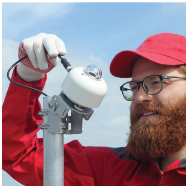
Figure2 PMF01 pyranometer mounting fixture can be used for easy installations of a pyranometer, in this case SR30, in Plane of Array for PV system performance monitoring and meteorological applications
