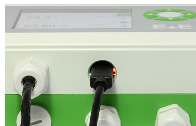
Fig. 28 Plugged USB cable and LED indication
